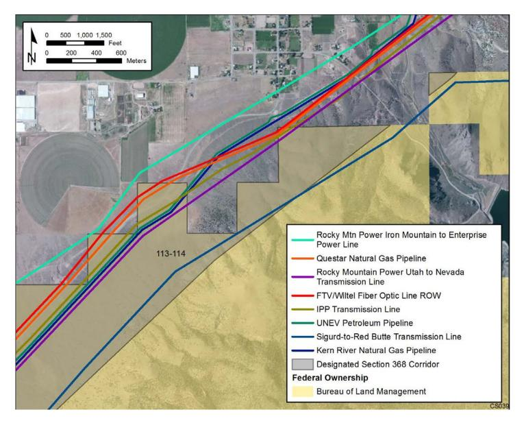
FIGURE 3-19 Detail of Congested Section of Corridor 113-114
