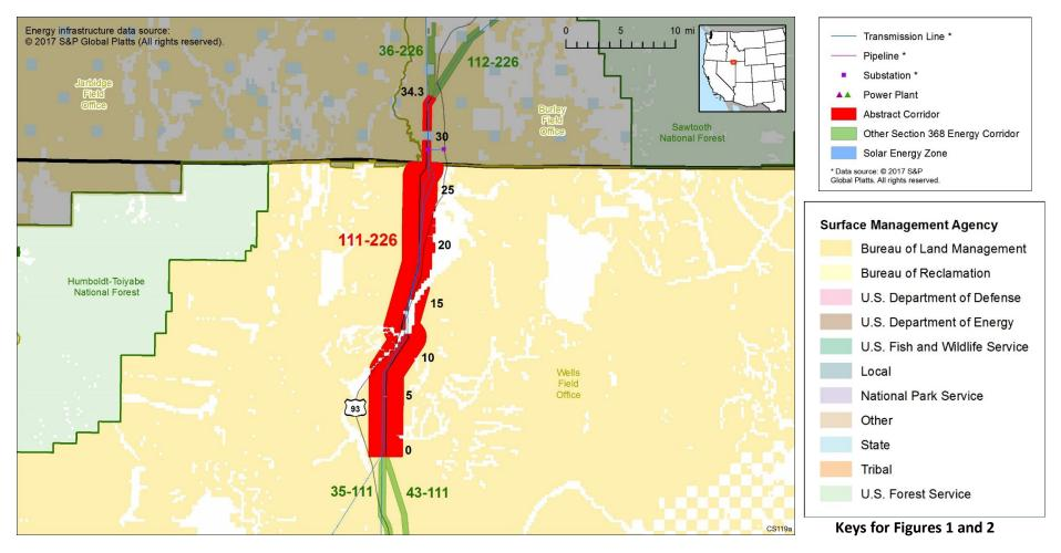
Figure 2. Corridor 111-226 and nearby electric transmission lines and pipelines (grayed out area outside of Region 2 and 3 Review)
