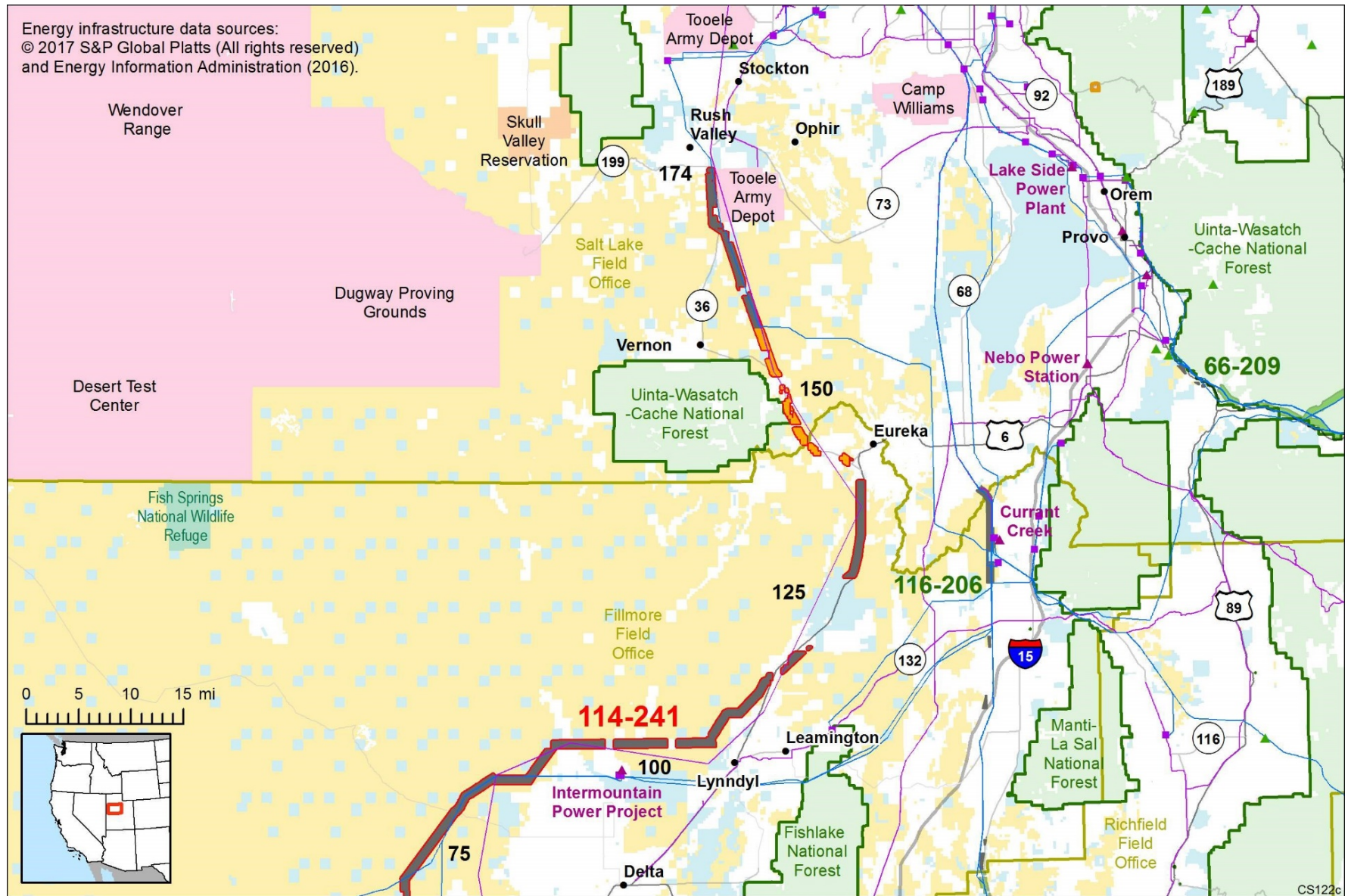
Figure 3. Corridor 114-241 (MP 75 to MP 174) and nearby electric transmission lines and pipelines
