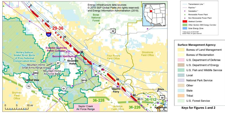
Figure 2. Corridor 29-36 and nearby electric transmission lines and pipelines
