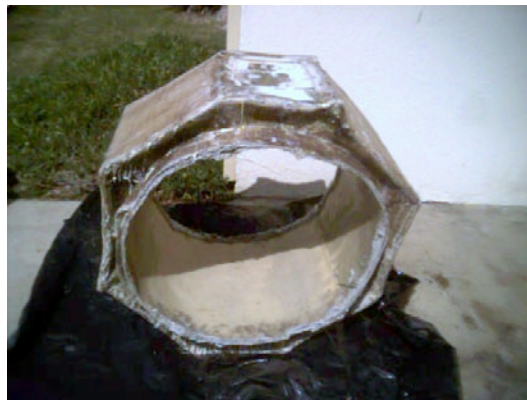
FIGURE 5. CONCRETE PIPE AFTER 9% DIA. DEFLECTION TEST
