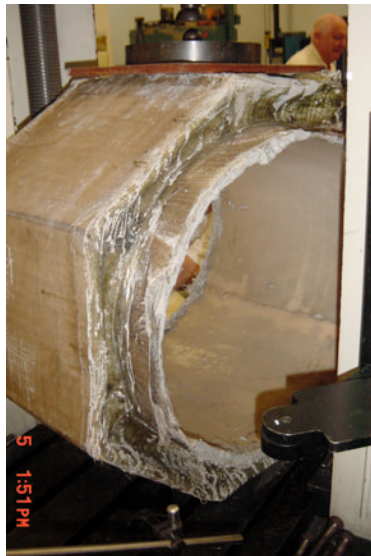
FIGURE 4. CONCRETE PIPE TESTED TO 9% DIAMETER DEFLECTION
