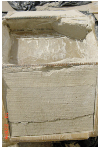
FIGURE 7. VIEW OF CRACKED CONCRETE PIPE SIDE WALL
