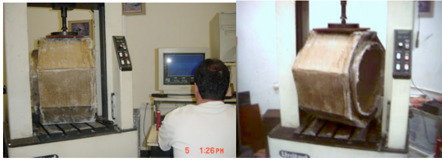
FIGURE 3. BEGIN TESTING CONCRETE PIPE TO 9% DIA. DEFLECTION
